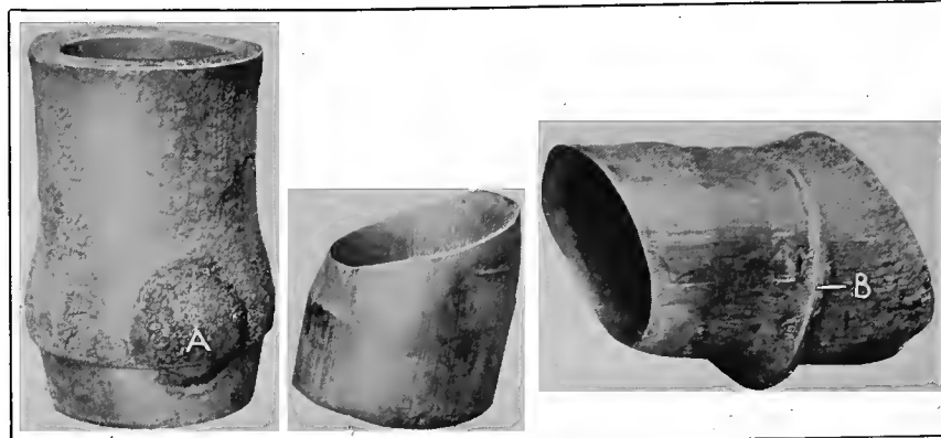
FIG. 19. EXAMPLES OF SPOILED FORGINGS
